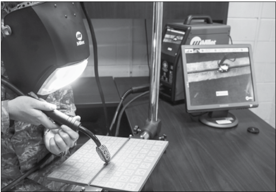
Airman 1st Class Taylor Dow, 7th Equipment Maintenance Squadron metals technology apprentice, uses the augmented reality welding system to train on welding a groove well Aug. 5 at Dyess Air Force Base, Texas.
